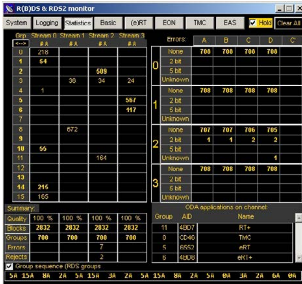
Figure 9 - 8 shows the RX014 statistics window. An overview is given of all received data expressed in number of blocks, groups or in percentages. The type of errors are reported and in case of RDS2 tunneling RDS data (as in the picture above) the group types in each stream are shown. Most of the known ODA Application IDs (AID) are shown together with the groups where the respective data may be found. At the bottom of the window the sequence of the received groups is shown.
