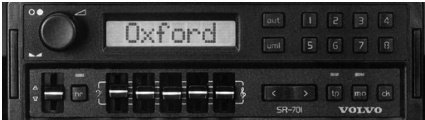
The first commercial RDS car radio on the European market was the Volvo SR-701 in 1987.
